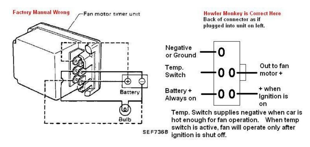
Some people will just ground temp. switch lead to ensure fan operates for 17 minutes every time car is shut off.
