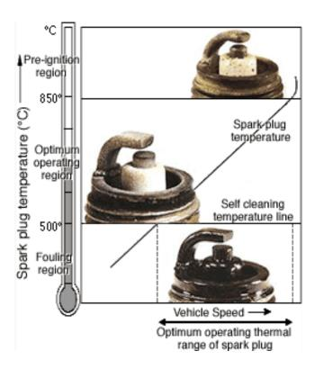
The firing end appearance also depends on the spark plug tip temperature. There are three basic diagnostic criteria for spark plugs: good, fouled and overheated. The borderline between the fouling and optimum operating regions (500&def;C) is called the spark plug self-cleaning temperature. The temperature at this point is where the accumulated carbon and combustion deposits are burned off.
