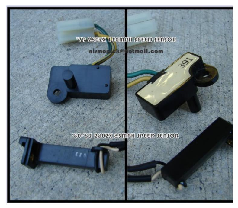
If you still have the 85mph speedo, you'll see how the speed sensor is attached. Just remove the one from the 130mph and install the 85mph one.
