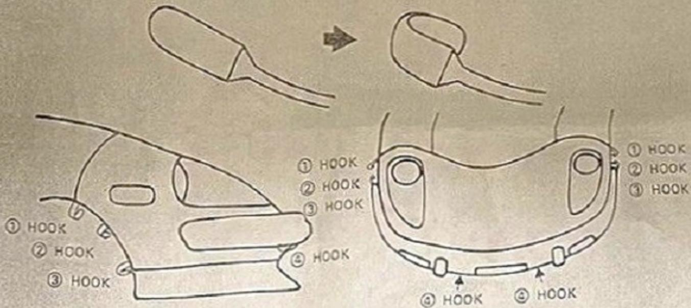
Securing hooks 1, 2 and 3 are attached to the leading edges of the front fender lips. Securing hook 4 is attached to the trailing edge of the front bumper underside. Secure bra material behind bumper guards.
