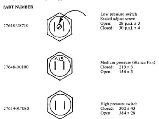
A letter and number, A-5 for example, indicate the production date, except on the medium pressure switch where A15 is the identification number. To identify the low pressure switch, look for the screw in the center. To identify the medium pressure switch, look for the number A15. The high pressure switch lacks either identification.
