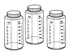
This kit provides three, 12 ounce plastic bottles and related fittings to replace the existing 7 ounce bottles. These bottles will accommodate the proper lubricant charge when retrofitting from R-12 to R-134a refrigerant systems.
