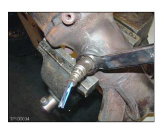
2/6 NTB10-009b 1. Clamp the exhaust manifold/catalyst/front tube in a vise.
