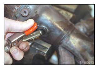
14. If metal debris remains trapped in the boss threads, use a spiral nylon brush to remove it.
