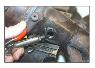
4/6 NTB10-009b 10. If metal debris remains trapped in the boss threads, use a spiral nylon brush to remove it.
